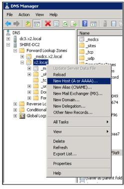
2 In the New Host dialog box, enter wcm under Name and provide the IP address of the IIS Server.
